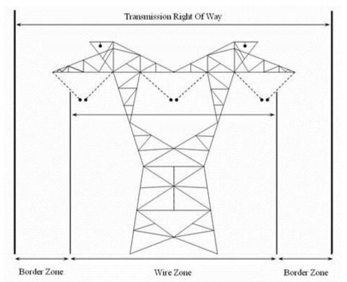
\* The wire zone is the area directly under the conductors and extending 15' on each side; the border zone extends from this point out to the edge of the right-of-way.
